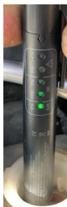
Figure 4.brake fluid test with Testboy 50.
